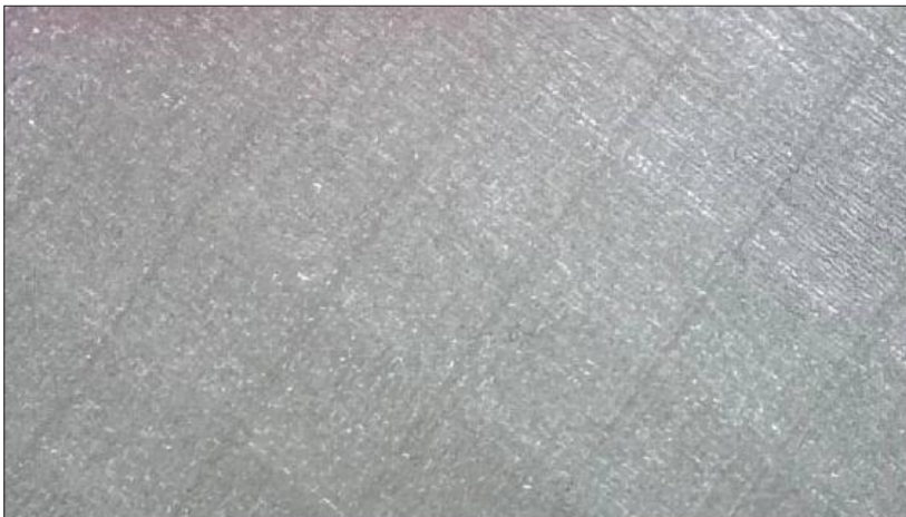
Fig (8): Microscopic image of the first model showing a 20% fill rate.
