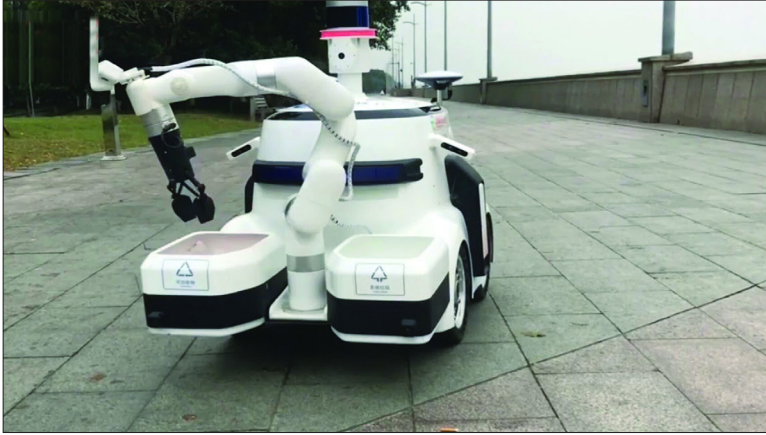
Figure 4: Robot collecting and sorting waste
