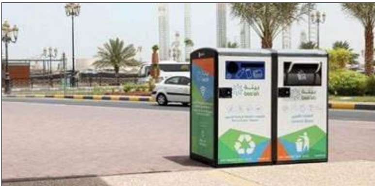
Figure 5: Smart, internet-connected, solar-powered waste containers
